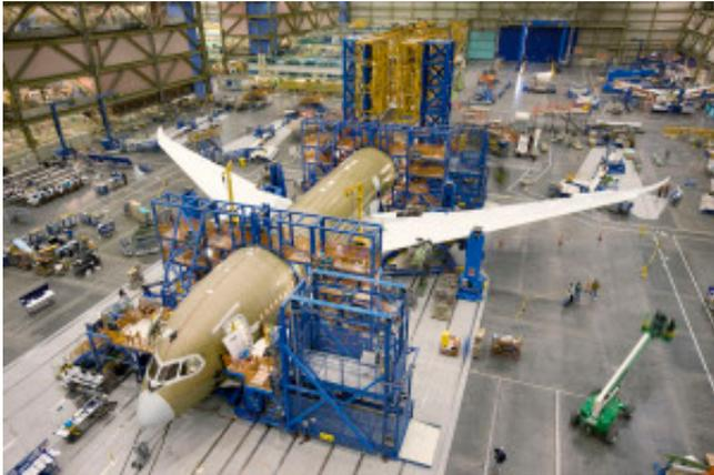
Aerospace automation provider Advanced Integration Technology incorporated Safety PLCs, Motion Control, plus safety and standard I/O, all on a single PROFINET network for more efficient, compliant automation. As a prime contractor on the Boeing 787 Dreamliner, AIT had responsibility for the final assembly and body join functions, charged with delivering a fully automated positioning and joining system.
