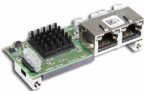
Protocol (MRP) and Isochronous Real-Time protocol (IRT), the comX 51 CA-RE passed PI's tests for the highest Conformance Class C as well as the highest Netload Class III. Typical applications for Class C PROFINET IO include high-speed, synchronized systems such as motion control. Netload Class III requires the device to exhibit advanced robustness even under the highest traffic densities as defined by the PI Specifications.
