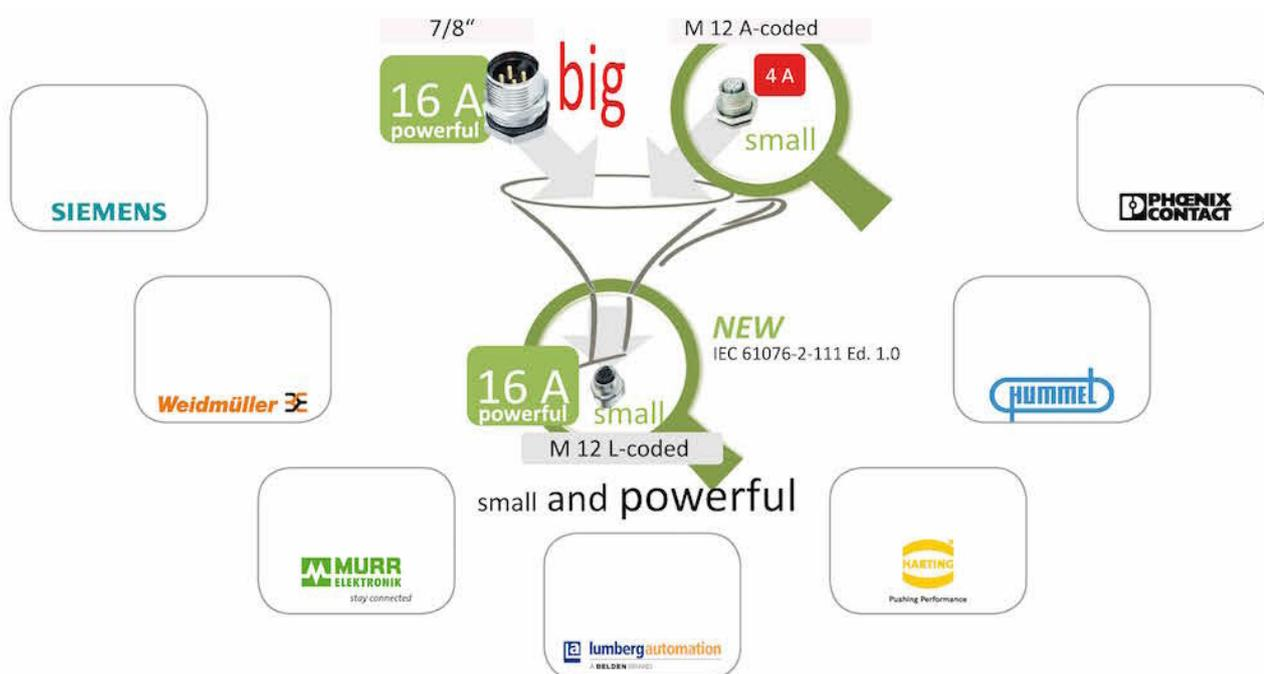
In the context of Industrie 4.0 this step also makes sense as it saves significant space on the device and in the installation compared to the 7/8" plug connector. The M12 L-coded is thus also a decisive step forward for miniaturization. The M12 L-coded is currently being internationally standardized and is already being offered by many connector manufacturers.
