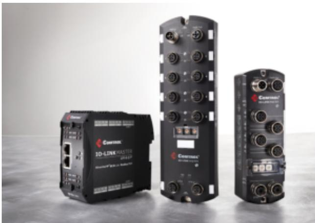
Control's MultiLink technology allows IO-Link Masters to simultaneously provide sensors Process data to PLC platforms, while also sending the sensors ISDU Service and Process data via OPC-UA upstream to IIoT/Industry 4.0 Cloud solutions or factory SCADA systems. Control's IO-Link Masters are available with PROFINET, which is capable of running OPC UA with MultiLink.
